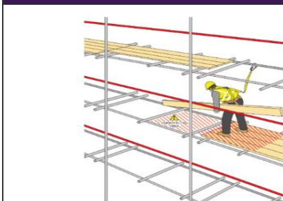
Example of PFPE being used when lowering working platform boards
