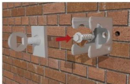
Example of a self-tapping screw being used with a welded plate.
