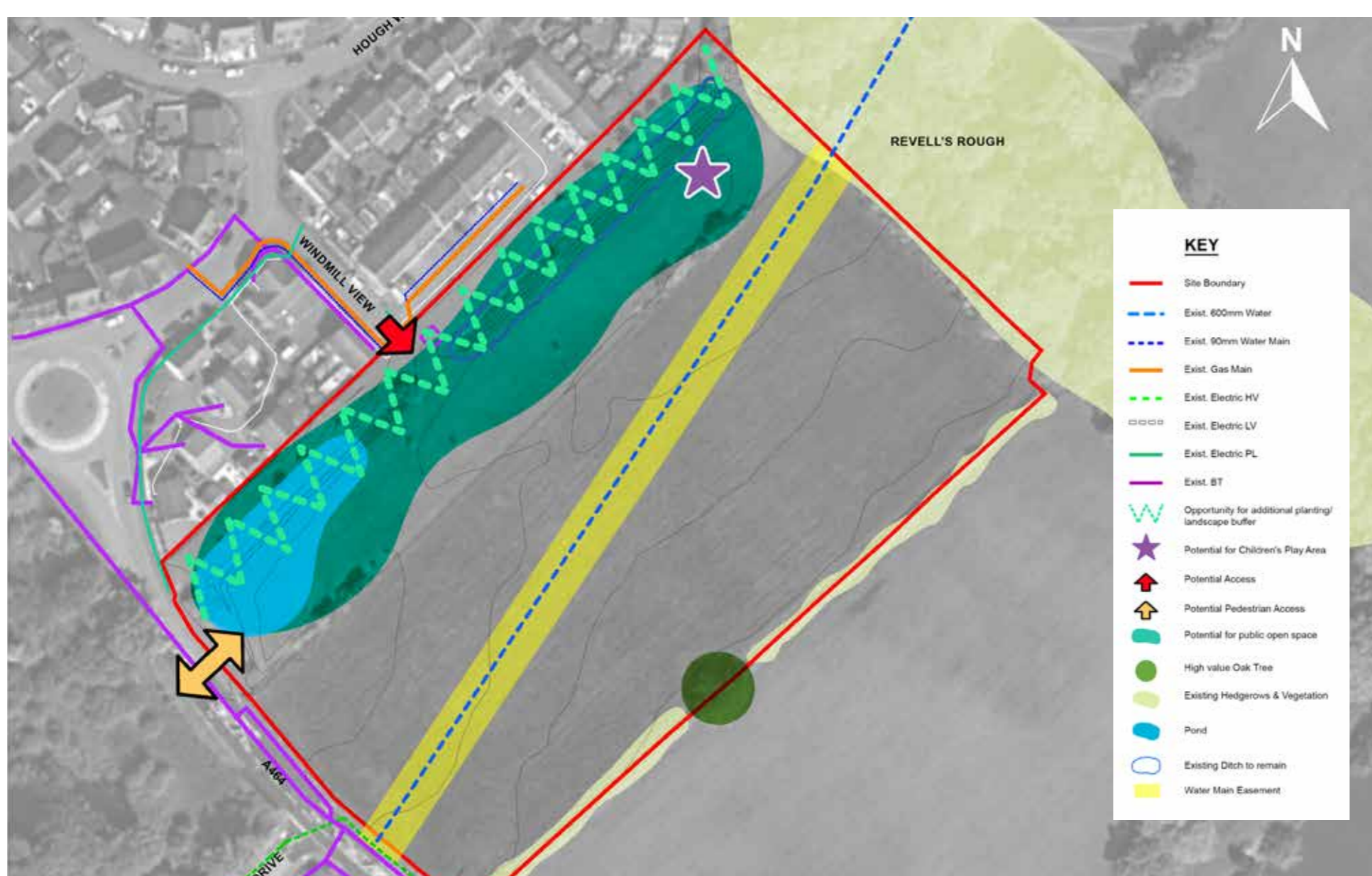
The Site's key constraints and our identification of opportunities to incorporate within our design proposals are illustrated in the drawing
