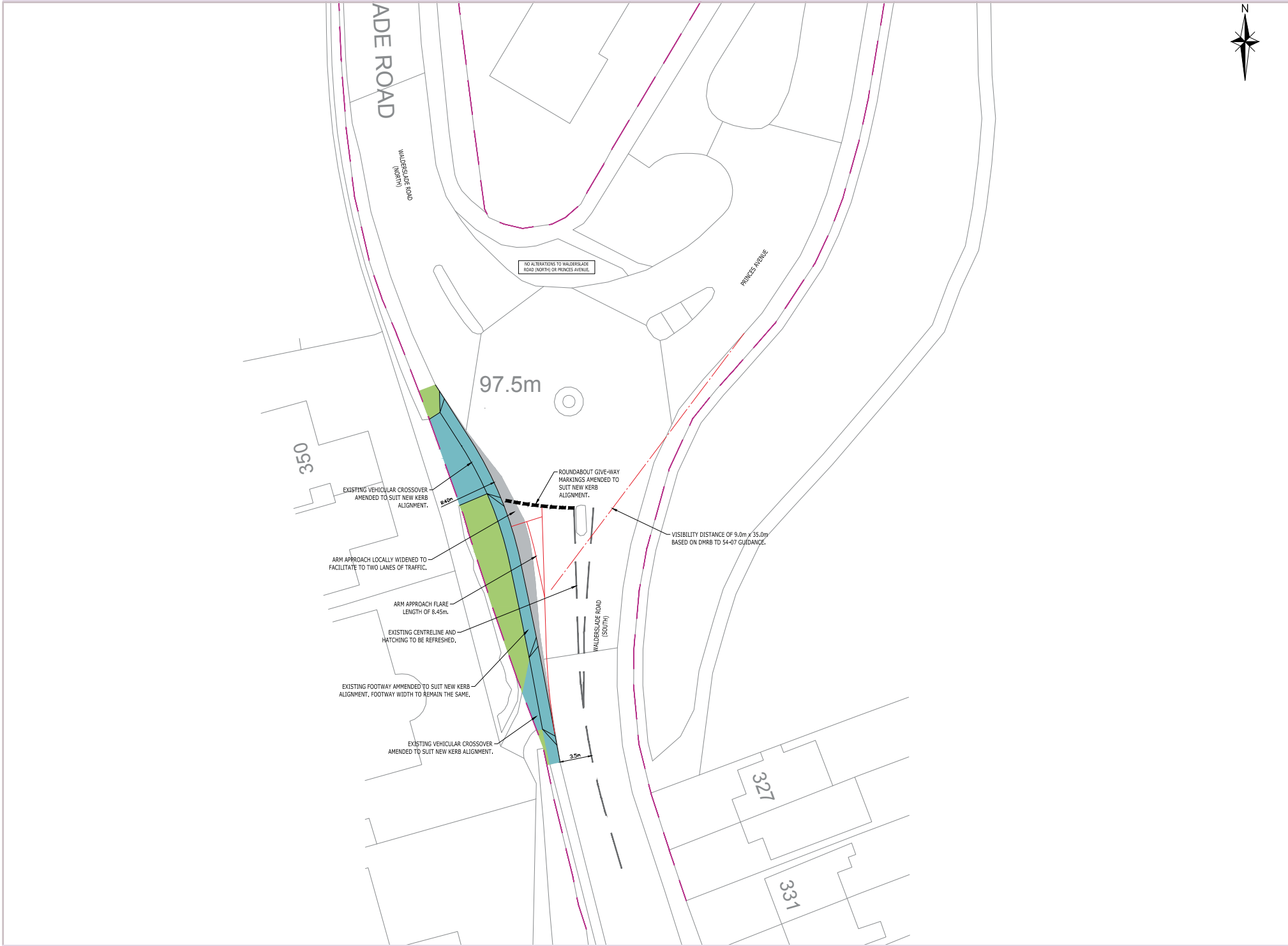
Princes Avenue/Prince Charles Avenue Roundabout – Widening of the approach from Prince Charles Avenue to facilitate two lanes of traffic.
