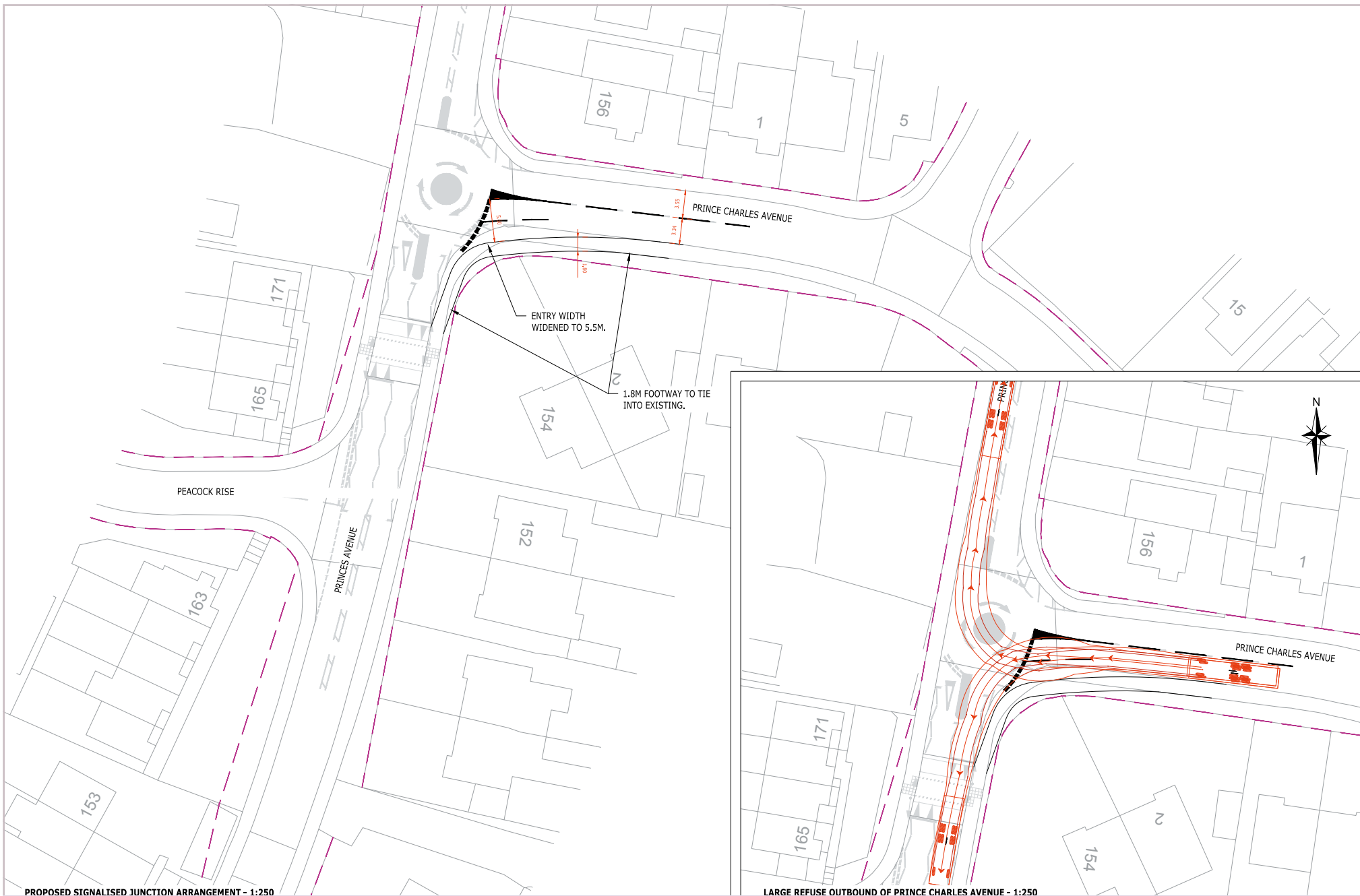
Princes Avenue/Prince Charles Avenue Roundabout – Widening of the approach from Prince Charles Avenue to facilitate two lanes of traffic.
