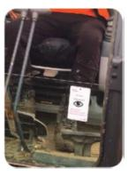
Plant Prompts must be provided to Excavator Operators prior to commencing works to remind them of the safety critical actions that help ensure the safe use of plant. (see section 2.2.5)
