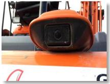
Rear view camera which must be kept in a fully operational state; and/or Convex mirror.
