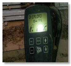
If capable of lifting more than 1000kg, the machine must have a Rated Capacity Indicator fitted to assist the driver to operate within safe limits by the use of audible and visual alarms.
