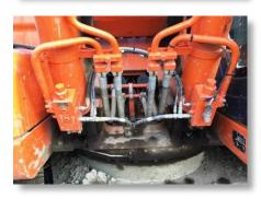
Check valves must be fitted when lifting more than 1000kg. These devices are fitted so that in the event of failure, it reverts to 'fail safe mode'; and
