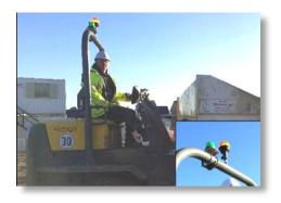
Dumper Operators must always wear a retractable seat belt to help ensure that they are held within the 'Roll-Over Protection System' in the event of overturning. All dumpers on TW Sites are to be fitted with a 'Seat Belt Warning System' consisting of:
