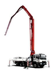
Lorry-mounted concrete pumps are used where concrete needs to be conveyed to large areas or areas that are difficult to access. The weight of laden machines can be very significant and therefore require similar checks and controls as with bringing a mobile crane onto site.
