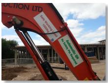
Appropriate Signage on the boom (i.e., safe working load);
