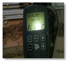
If capable of lifting more than 1000kg, the machine must have a Rated Capacity Indicator fitted to assist the driver to operate within safe limits using audible and visual alarms.
