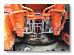
Check valves must be fitted when lifting more than 1000kg. These devices are fitted so that in the event of failure, it reverts to 'fail safe mode'; and
