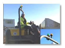
Dumper Operators must always wear a retractable seat belt to help ensure that they are held within the 'Roll-Over Protection System' in the event of overturning. All dumpers on TW Sites are to be fitted with a 'Seat Belt Warning System' consisting of:
