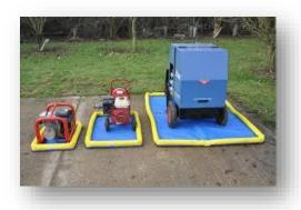
• A more effective alternative to standard drip trays is the 'Plant Nappy'. While containing any drips or spills of oil, the mat freely allows passage of water, such as rainfall, thus eliminating costly emptying of water filled contaminated drip trays after use.
