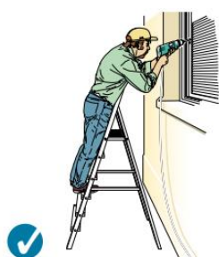
Figure 2b Correct - steps facing work activity
