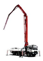
Lorry-mounted concrete pumps are used where concrete needs to be conveyed to large areas or areas that are difficult to access. The weight of laden machines can be very significant and therefore require similar checks and controls as with bringing a mobile crane onto site.
